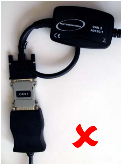
This cable combination with the CAN1 dongle in place will affect system communications
